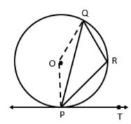
$m \angle OPT = 90^{\circ}$  (: radius is perpendicular to the tangent)
